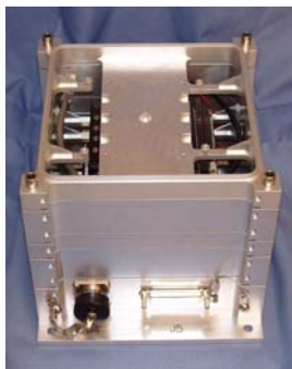
Electronics Stack with Integrated Heat Spreader
